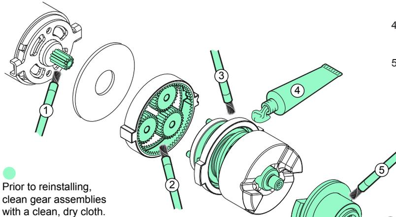
Prior to reinstalling, clean gear assemblies with a clean, dry cloth. Lightly coat all parts highlighted here with 'Y' grease. Apply a greater amount of grease to all internal and external gear teeth.
